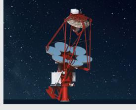
SST-2M ASTRI (image 2) and SST-2M GCT (image 3): both are dual-mirror designs that allow excellent imaging across a wide field of view with a short focal length. They use SiPMs in very compact cameras.
