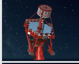
SST-1M (image 1): a single-mirror design with a camera that uses SiPMs and is a down-scaled version of the MST mount.
