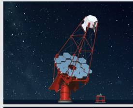
The SSTs will outnumber all the other telescopes and will be spread out over several square kilometers in the southern hemisphere array. This is because very high-energy gamma-ray showers produce a large amount of Cherenkov light, and the SST is sensitive to the highest energy gamma rays. The SST mirror will be about 4 metres in diameter and will have a large field of view of about 8-10 degrees. Three different SST implementations are being prototyped and tested:
