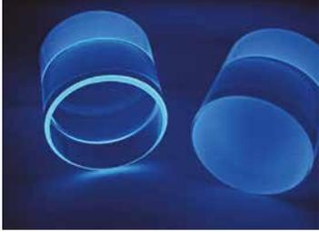
9 CRESST uses crystals of calcium tungstate to detect dark matter particles
