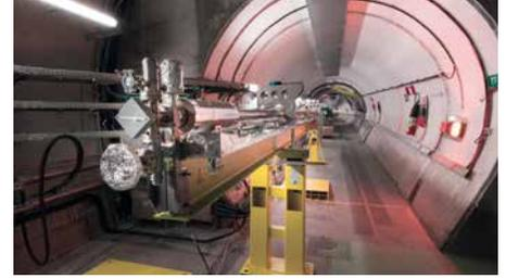
14 Key component of the AWAKE experiment: The 10-meter-long plasma cell
