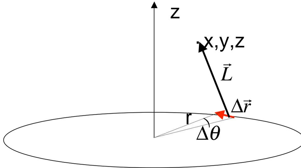
Magnetic field can be calculated analytically for points along the axis, but not for other points. Magnetic field will have components in all directions. Need to calculate them one at a time.
