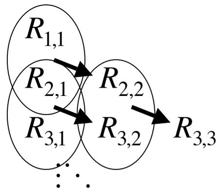
So, e.g., can get up  $h^6$  precision by extrapolating the trapezoidal rule calculations with spacing  $h, h/2, h/4$
