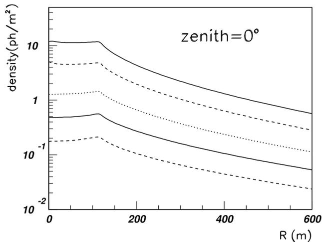
**Figure 2.4:** Radial Cherenkov photon density, for a vertically incident shower, at the MAGIC altitude of 2200 m above sea level. The profiles correspond (from top to bottom) to a gamma-ray energy of 100 GeV, 50 GeV, 20 GeV, 10 GeV and 5 GeV. The density is practically constant within a radius of 120 m from the shower axis (Cherenkov light pool), and falls off outside of it.
