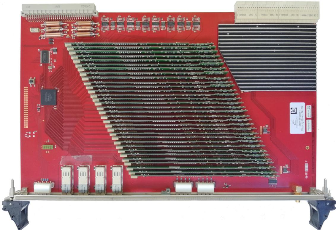
**Figure 2.11:** Clip-board №5 of the MAGIC-I Sum-Trigger-II unit. The board receives 32 single-pixel input signals from four multi-channel differential cables (lower left), and processes them with the delay modules visible in the center. The output signals are transferred to the sum-boards over the back-plane connection (upper right). A FPGA (left) controls the delay, attenuation and clipping settings. (G. Ceribella /MPI)
