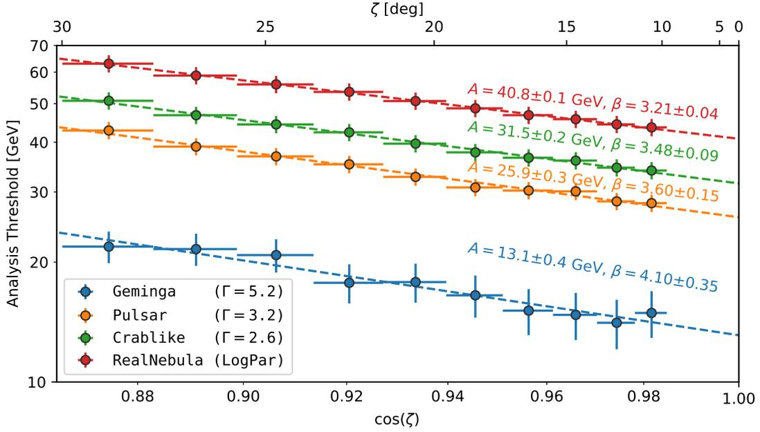
**Figure 4.24:** Energy threshold variation with the zenith distance  $\zeta$  of the observations, for several possible spectral sources. The threshold increases with  $\zeta$  due to the atmospheric absorption. The variation has been modeled as a power-law relation  $E_{\text{THR}} = A \cos(\zeta)^{-\beta}$  (dashed lines).
