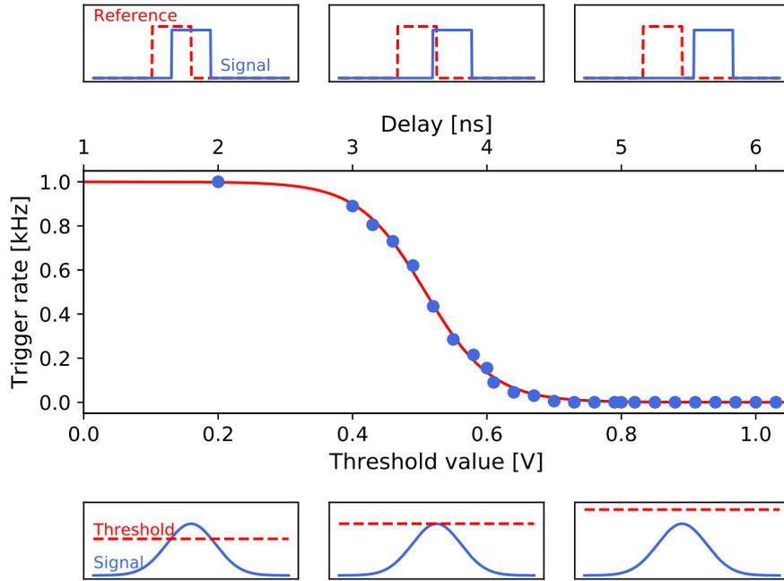
**Figure 3.1:** A sample rate scan for the attenuation values and the delays. In this figure, values on the x-axis can be interpreted either as voltage threshold values (bottom axis) or as delay values (top axis). Smaller panels show the relation between signals and the threshold value (for an attenuation scan) or the reference signal (for a delay scan) at various locations of the curve.
