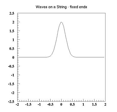
Initial pulse makes a big difference in which frequency components present The wavepacket is symmetric about the center. The Fourier components will be preserved in time, so we can see which are present at the start. Clearly, only the frequency components corresponding to standing waves which are symmetric about 0 will survive.
