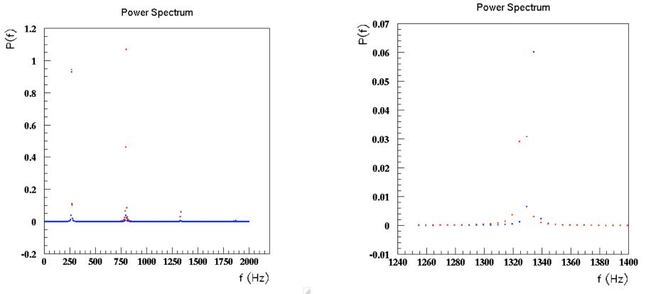
Dispersion is introduced in the stiff spring, because the effective wave speed becomes frequency dependent. The frequency components for the stiff string are shifted higher. Introduces characteristic sound. **Computational Physics I** Winter Semester 2006/
