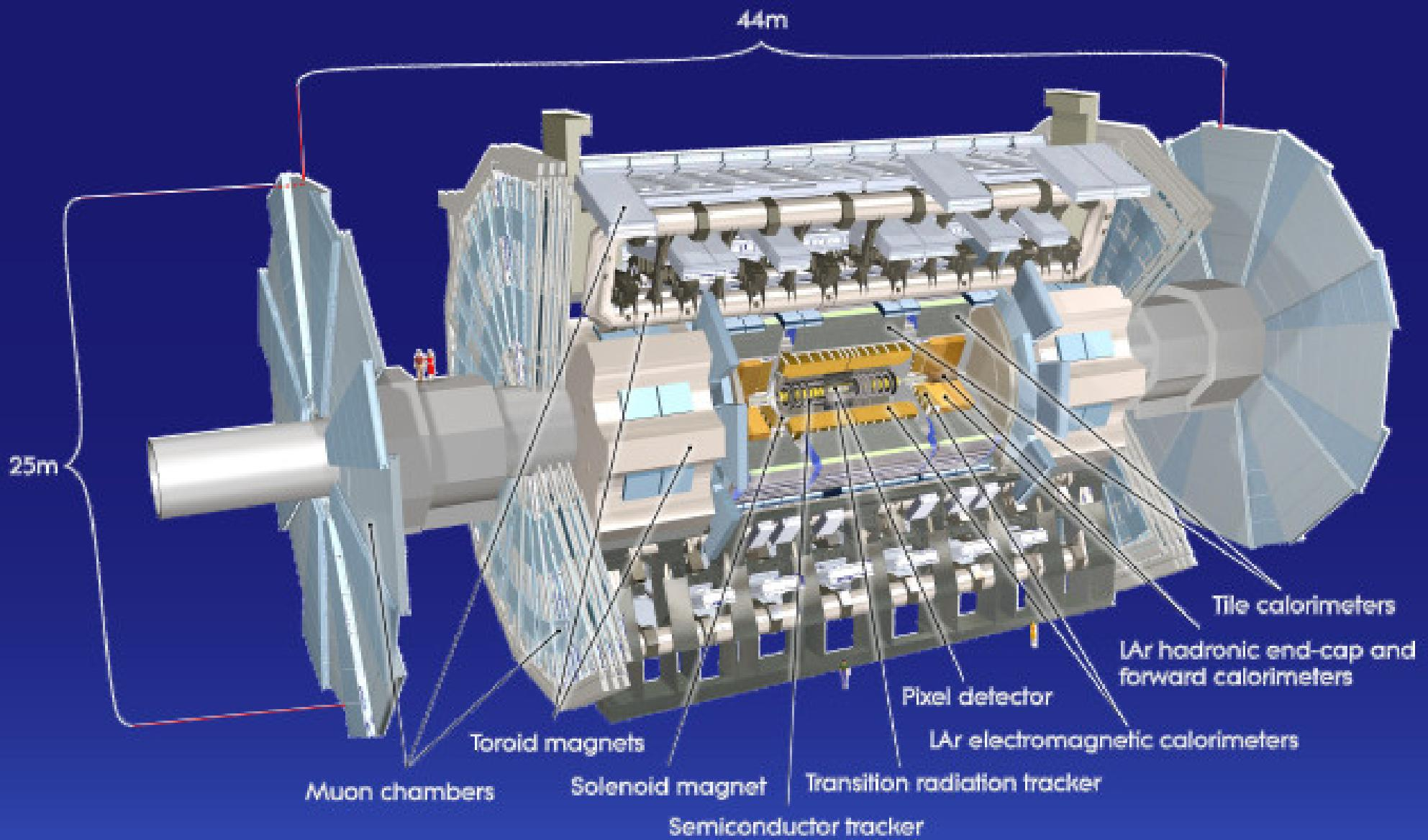
**A Torodial LHC ApparatuS:** 25 m high; 44 m long; 7000 t heavy
