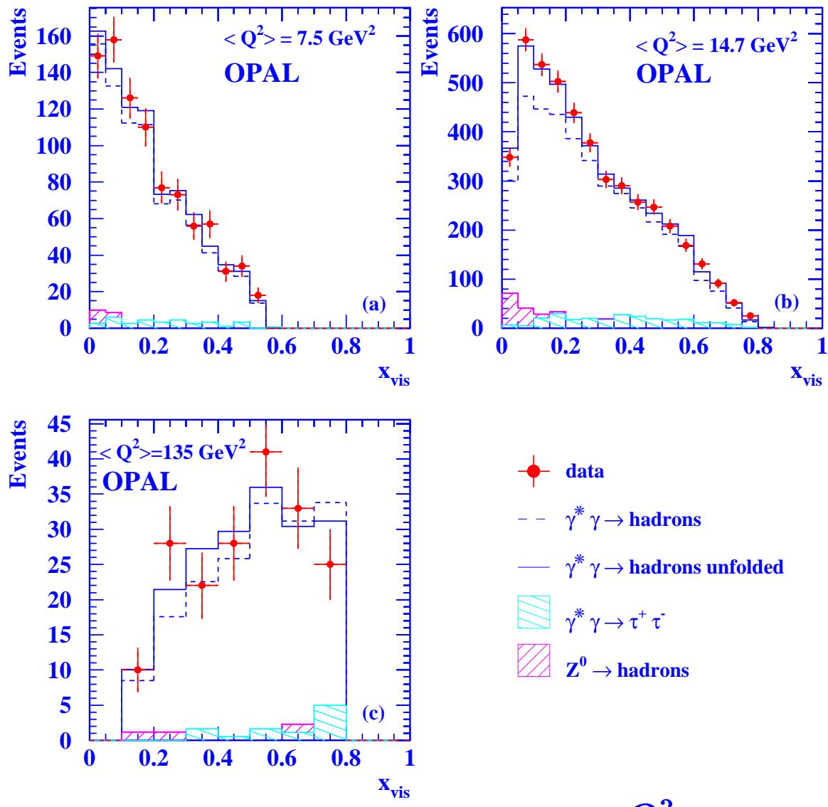
The mean  $x_{\text{vis}}$  increases with  $Q^2$
