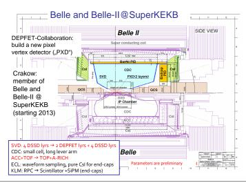
An upgrade for even higher luminosities with a new vertex detector is underway.
