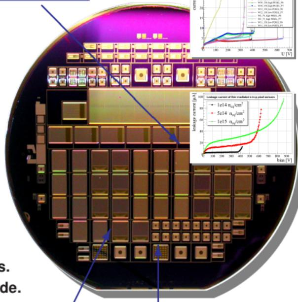
**Test structures:** Diodes, SLID
