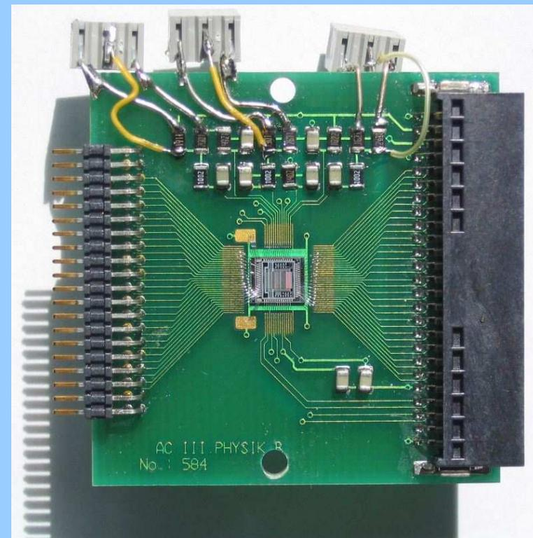
The preshape is bonded on a small board to perform tests.
