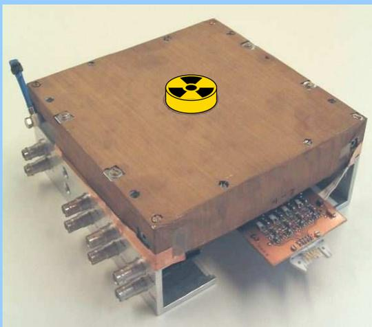
Test chamber,  $^{55}\text{Fe}$  source
