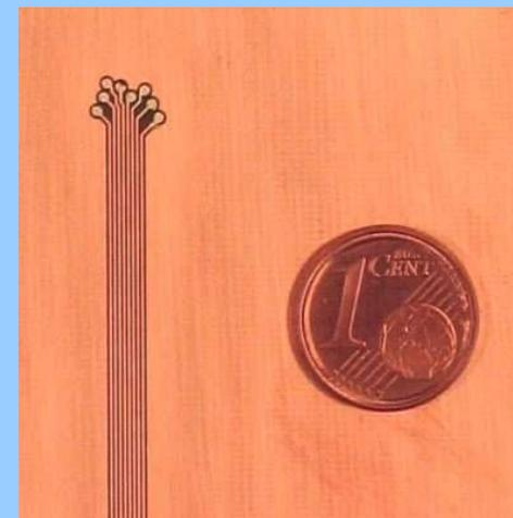
Anode strips,  $300\ \mu\text{m}$  pitch
