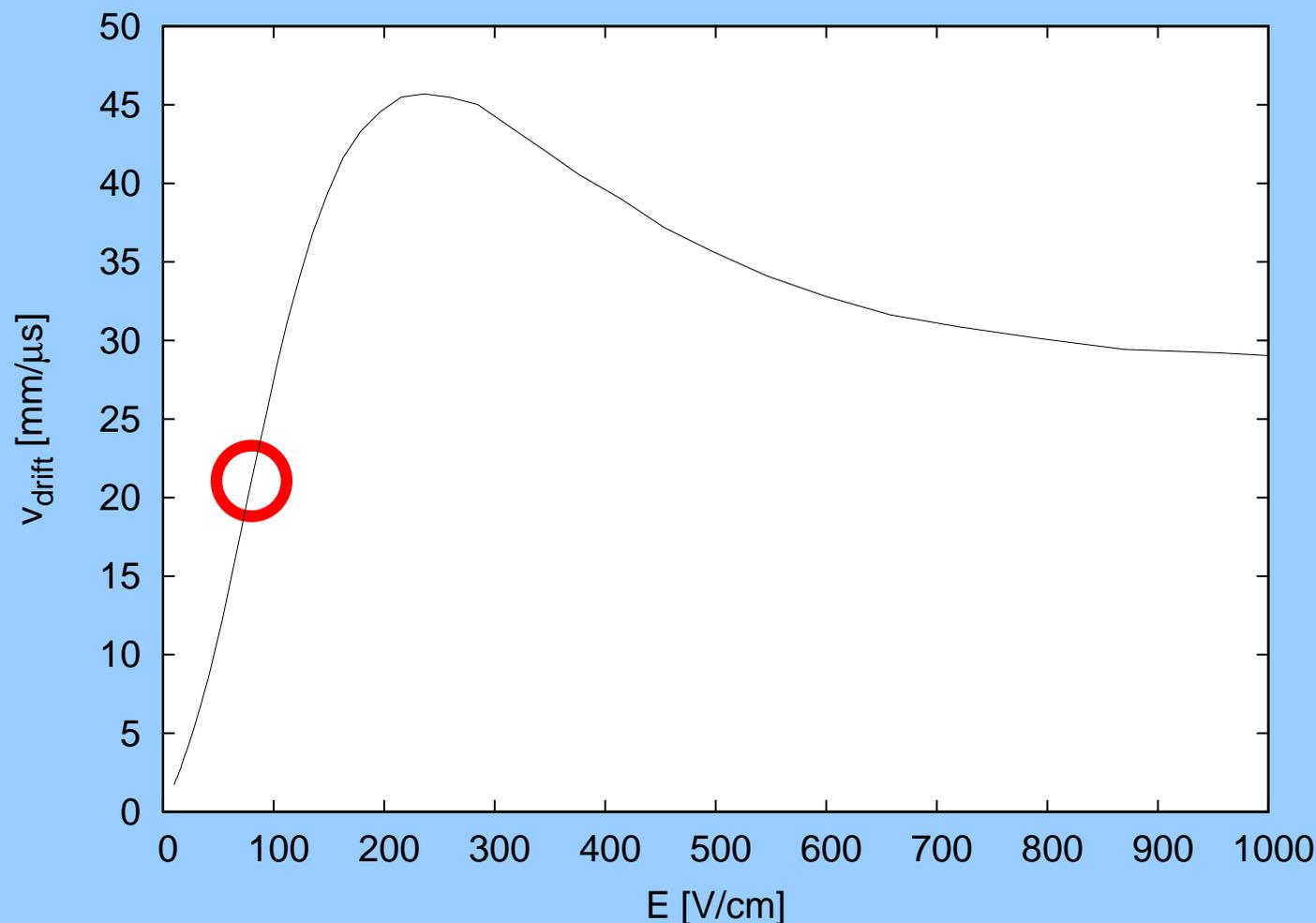
Maximal sensitivity at the steepest position (80 V/cm).
